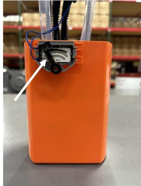
**STEP 11:** Install the SureFlo assembly into the tank, use caution with the float arm and do not over-rotate the pump once installed.
