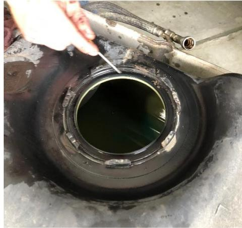
**STEP 10:** Install the fuel level float arm onto the SureFlo assembly by gently clipping the arm into the fuel level sensor.
