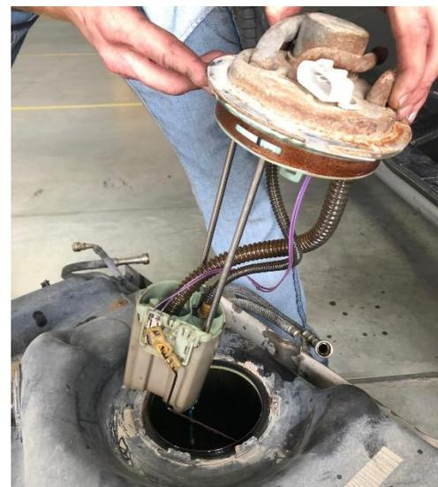
**STEP 9:** Clean all debris from around the o-ring groove and tank sealing surface. Place your new o-ring included with the SureFlo onto the top of the tank.
